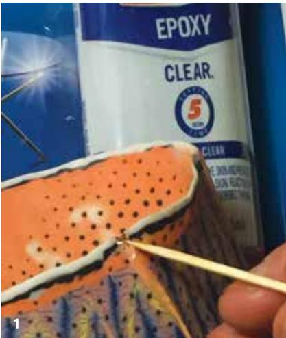
1 Mix the five-minute epoxy, then immediately apply it to the crack with a toothpick.
